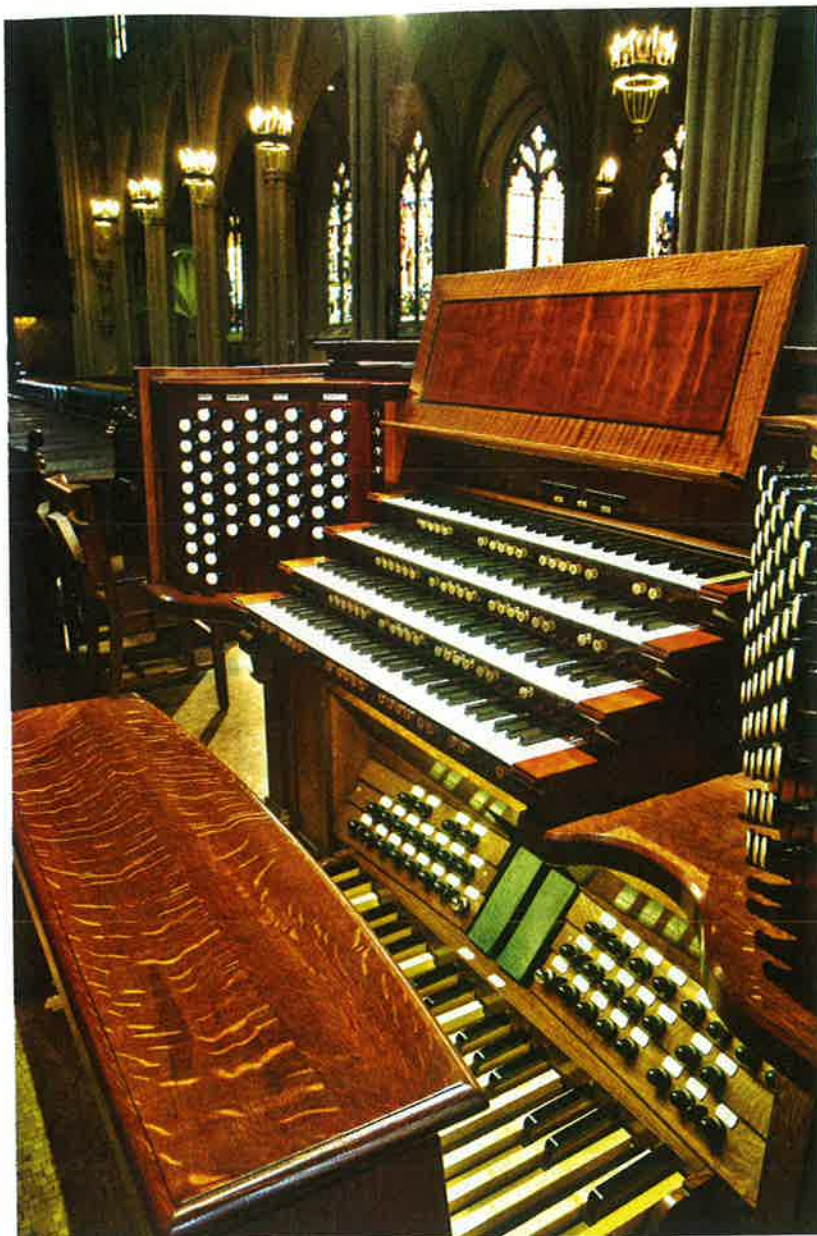
Console (detached and reversed; bone keys with Gabon ebony sharps) (photo: Robbie Lawson)
